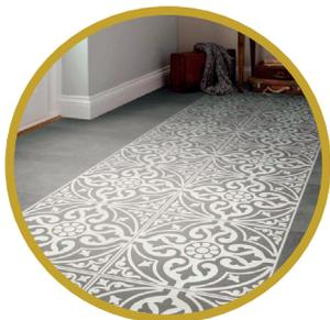
Possibly the best floor finish for use as the underfloor heating will gently warm the surface. Tiles/Stone/Slate are low in height and great at conductivity. UFHN LTD recommends this floor finish to achieve optimum results from your system. We would advise a small expansion gap is left around the perimeter of the room, filled with a flexible sealant.
